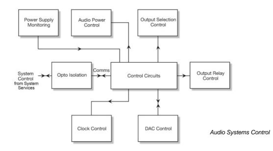
The Microcontroller (PIC) is in sleep mode during audio playback. The Microcontroller is woken by communications from the System Services Board to control the de-jittering circuits and DAC.
