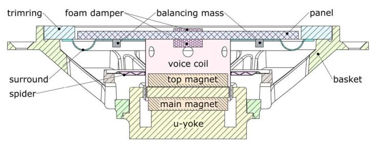
Fig. 9 Cross-section view of Balanced Mode Radiator.
