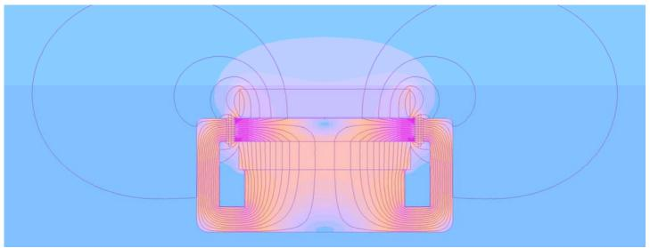
Fig. 10 Flux density plot of BMR magnet system
