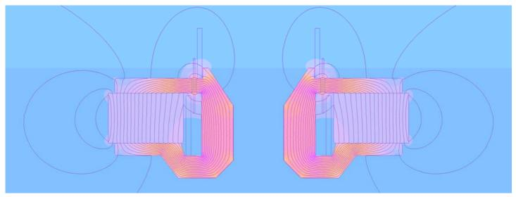
Fig. 13 Flux density plot of 8" Naim woofer.
