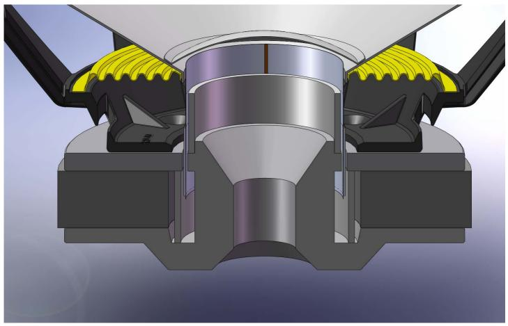
Fig. 14 Coss-section of Ovator S-600 Bass Driver
