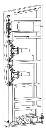
Cutaway drawing of the Ovator S-400 cabinet. Features of note include the isolated BMR module, separate enclosures for the two bass drivers and the provision of controlled 'leaks' between the latter and the external air
