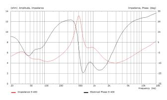
Impedance modulus (red trace) and phase (black trace) versus frequency
