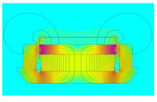
FEA model of the S-400 BMR driver magnetic circuit showing the even flux density achieved in the magnet gap
