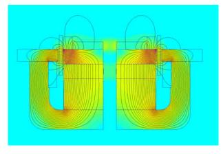
FEA model of the S-400 bass driver magnetic circuit showing the even flux density achieved in the magnet gap
