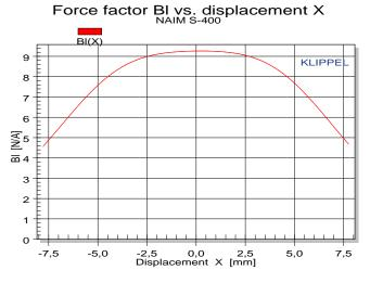
Klippel Analyzer measurement of the linearity of the S-400 bass unit's motor
