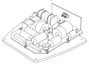
Suspended from the plinth to isolate it from vibration, the crossover module combines careful layout with meticulous choice of components
