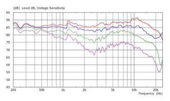
On- and off-axis response of a typical two-way system
