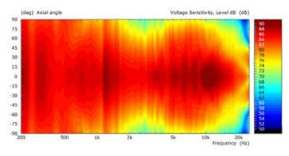
Directivity plot of a typical two-way system
