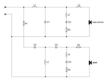
Circuit schematic of the Ovator S-400 crossover. Acoustic slopes are 4th-order Linkwitz-Riley to ensure that the drivers remain in phase throughout the crossover region
