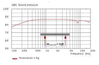
Figure 2. Free disk driven at the first nodal line by an ideal, mass-less force
