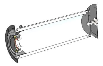
Cross-section of the S-800 BMR in its mechanically isolated aluminium cylinder
