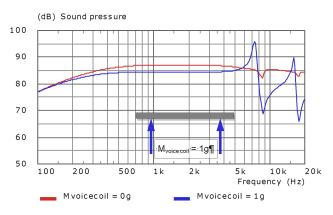
Figure 3. When a motor with finite mass is substituted, the natural balancing of the disk is lost (blue curve)
