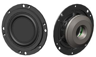
Front and rear views of the S-800's new 82mm BMR. Key features include a larger, 55mm diameter voice coil and generous rear venting through the neodymium ring magnet
