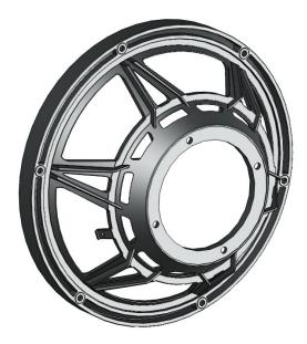
Triangulated structure of the bass driver chassis combines high stiffness with free air flow from the back of the diaphragm and suspension
