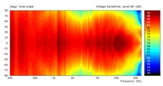
Figure 6. Sound pressure level versus frequency versus angle for the same two-way speaker as Figure 5
