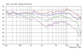
Figure 5. Sound pressure level versus frequency for a two-way speaker at horizontal angles of 0° (on-axis, red), 30° (blue), 60° (green) and 90° (purple)
