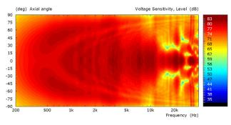
Figure 8. Sound pressure level versus frequency versus angle for the S-800 BMR. Contrast this with Figure 6
