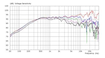
Figure 7. Sound pressure level versus frequency for the S-800 BMR at horizontal angles of 0° (on-axis, red), 30° (blue), 60° (green) and 90° (purple). Contrast this with Figure 5
