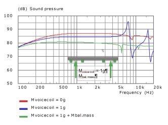
Figure 4. Adding balancing masses restores the behaviour of the free disk (green curve)
